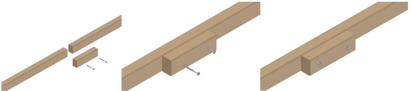
The outer support beam should be mounted circa 6 cm within the outer edge of the paving stones. All other support structure beams should be placed in the middle of the paving stones and fixed in place with brackets. A spacing of at least circa 10 mm from house wall or other structures must be observed.
