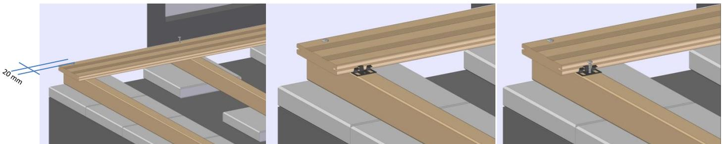
For the second row of decking boards cut the decking board in such a way that the board lies on at least two support beams. The same must be done for the last decking board on the other side of the decking. Insert the complete row of decking boards into the clips and screw the clips firmly to the support structure beams.
